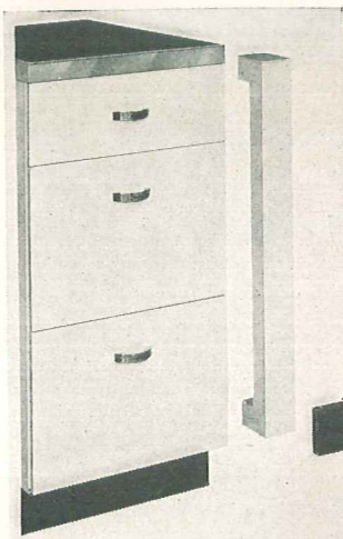
BASE SCRIBING FILLER—Designed to take up any left over space 3" or under. Can be cut on job to fit uneven walls.
